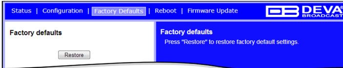
To restore DB90-TX to its Factory Defaults you should first press the Restore button. A new window will appear: confirm that you want to restore factory defaults and wait for the process to complete. All settings will be restored to their factory defaults except for
