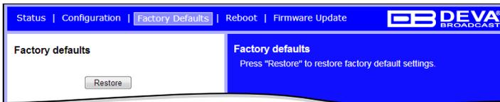
To restore DB90-RX to its Factory Defaults you should first press the Restore button. A new window will appear: confirm that you want to restore factory defaults and wait for the process to complete. All settings will be restored to their factory defaults except for
