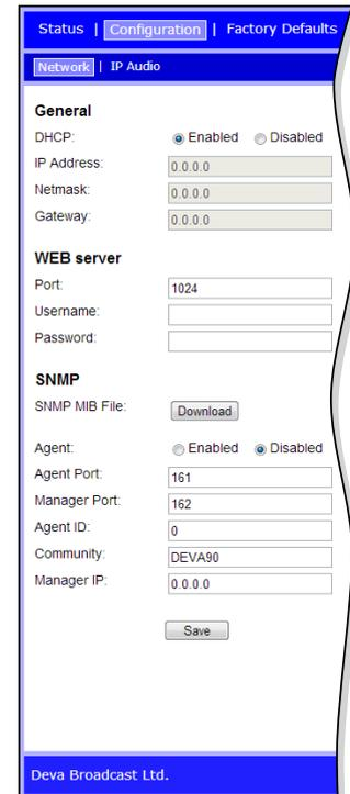
The screenshot shows the 'Configuration' tab with 'IP Audio' selected. Under 'General', DHCP is 'Enabled', and IP Address, Netmask, and Gateway are all '0.0.0.0'. Under 'WEB server', Port is '1024', Username and Password fields are empty. Under 'SNMP', 'SNMP MIB File' has a 'Download' button, 'Agent' is 'Disabled', 'Agent Port' is '161', 'Manager Port' is '162', 'Agent ID' is '0', 'Community' is 'DEVA90', and 'Manager IP' is '0.0.0.0'. A 'Save' button is at the bottom.
